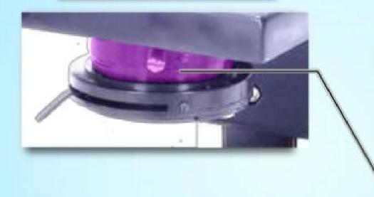
The lens under the stage that <u>focuses light</u> from the illuminator through to the <u>hole</u> in the stage.
